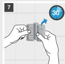
7 Place the accessory on the wall from the bottom, remove the item and press for 30".
