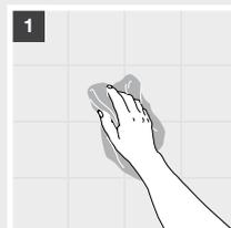
1 Clean the mounting surface with a 50% water and alcohol solution.
