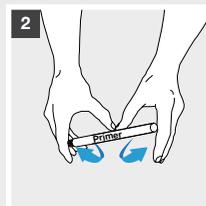
2 Tighten the "first" tube to break the inner capsule until the liquid soaks the cap.
