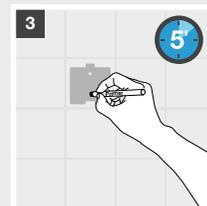
3 Apply a thin layer of the "first" tube on the surface of the support and on the wall to increase the adherence and let it act for 5 minutes.
