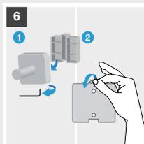
6 Assemble the support on the accessory and remove the adhesive protection. Do not touch with your fingers.
